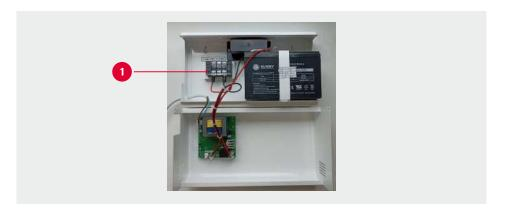
3.) Press the **"ON" switch** 1 - the device will activate within approximately 3 seconds. The system will operate and the emergency lights and status LED will indicate "ON."
