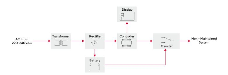
Principle of Operation - Central Battery Systems: 12V Series
