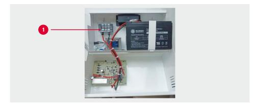
3.) Press the R or L switch 1 to activate the control unit. The device will supply electricity from the battery to the emergency light.
